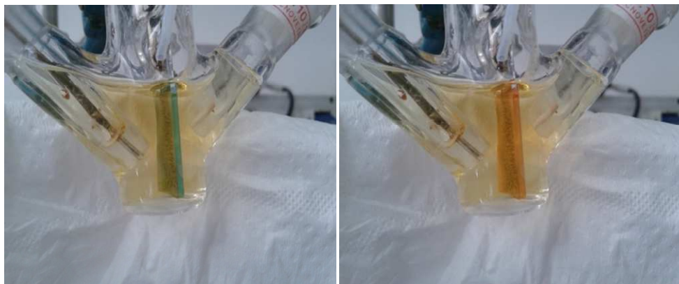
Figure 58. Electrochromism of the (T8) 3 oligomer on ITO working electrode (on the left: oligomer doping, on the right: oligomer undoping)
