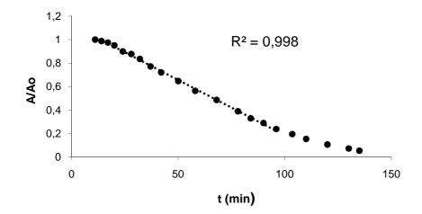
*Figure 36.* Zero-order kinetic with respect to the aryl azide in the range of A/Ao between 1 and 0.3.
