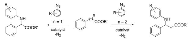
Scheme 63. Synthesis of  $\alpha$ - or  $\beta$ -amino esters by the benzylic amination reaction.
