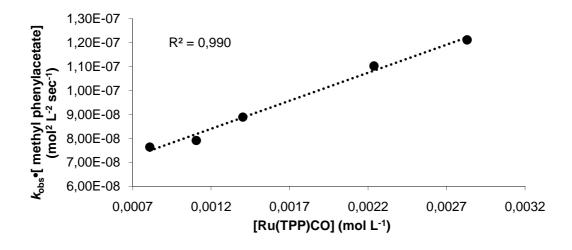
*Figure 37. First-order kinetic with respect to Ru(TPP)CO concentration.*
