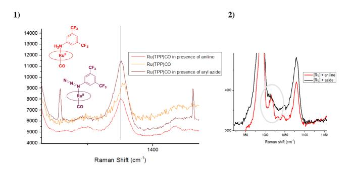
*Figure 16. 1) Ru*(*TPP*)*CO* oxidation marker band shifts upon coordination of an axial ligand. 2) *Coordinated aryl group band in the spectra of complex 15 (red line) and of Ru*(*TPP*)*CO in the presence of 38*(*black line*).
