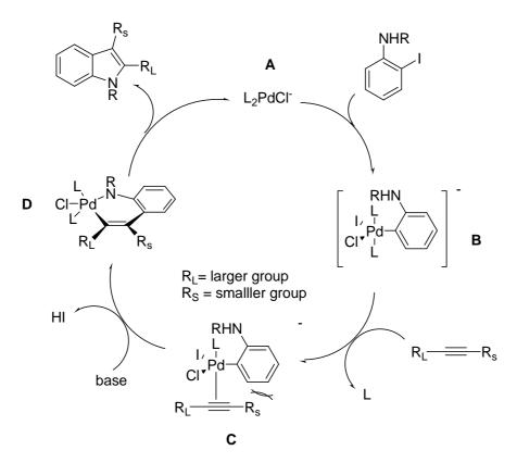
Figure 14. Mechanism for the Larock heteroannulation.
