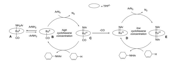
Scheme 57. Catalytic cycle proposed for allylic amination catalysed by Ru(TPP)CO.
