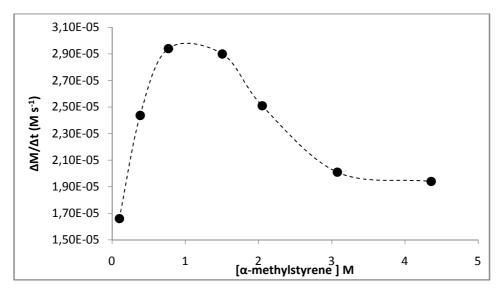
Figure 35. Plot of the reaction rate versus styrene concentration.
