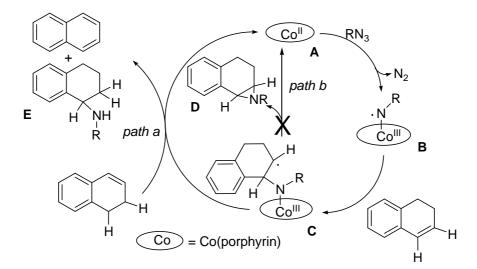
Scheme 54. Mechanistic proposal for dihydronaphthalene amination.
