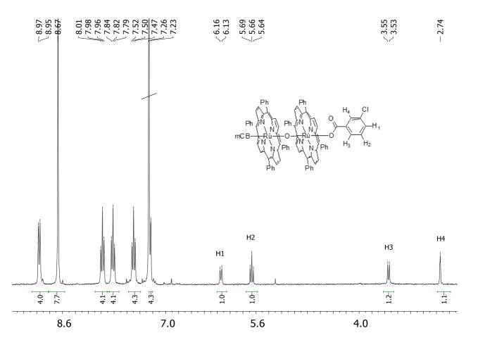
**Figure 28.** <sup>1</sup>*H* NMR spectrum of complex **91**, typical pattern for  $Ru(TPP) \mu$ -oxo complexes is observed in the aromatic region, highly shielded protons of the benzoate moiety were detected between 6.5-2.5 ppm.
