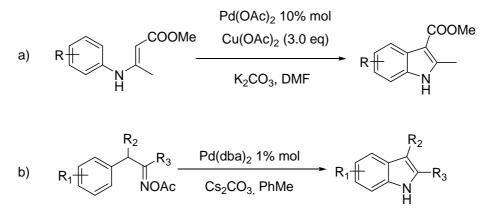
Scheme 46. Indole synthesis developed by a)Glorius and b)Hartwig.
