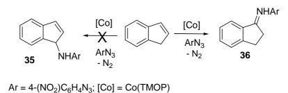
Scheme 56. Reaction between indene and 4-nitrophenyl azide in the presence of Co(TMOP).
