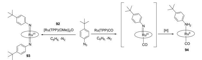
Scheme 76. Reaction between 4-tert-butylphenyl azide and ruthenium complexes with different oxidation state.
