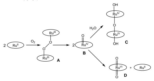
Scheme 7. Mechanism of oxidation of Ru(II) porphyrin complexes by dioxygen.
