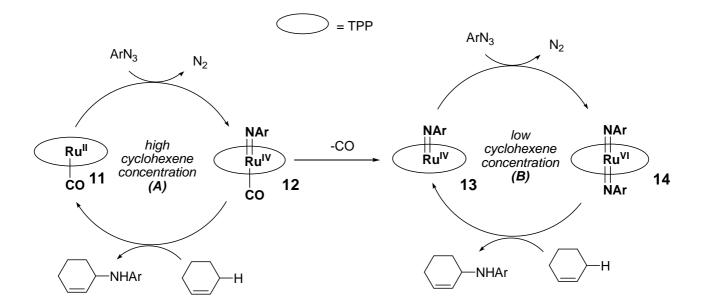
Scheme 32. Mechanism of Ru(TPP)CO-catalysed allylic amination of cyclohexene.
