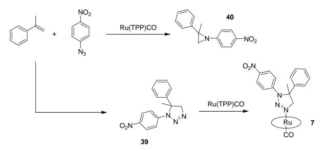
Scheme 58. Ru-catalysed and uncatalysed reaction between  $\alpha$ -methyl styrene and 4-nitrophenyl azide.
