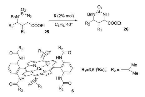
Scheme 40. Co-catalysed intramolecular C-H amination to give cyclic  $\alpha$ -amino ester.
