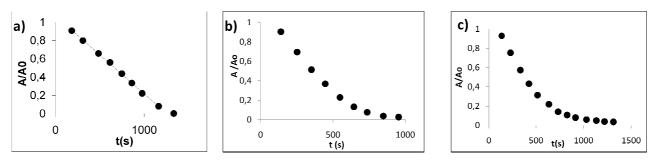
Figure 19. Aryl azide consumption monitored by IR spectroscopy at [styrene] = 0.1 M(a), 2.1 M (b), 3.0 M (c).
