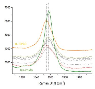
*Figure 18.* Time resolved spectra of the catalytic mixture in the oxidation marker band region, the pale red line is the first spectrum acquired, the pale green is the last acquisition. The bold lines are the reference spectra of Ru(TPP)CO and the bis-imido complex 10.
