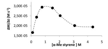
Scheme 60. Plot of the reaction rate versus  $\alpha$ -methyl styrene concentration.
