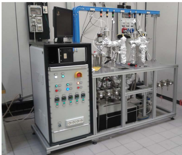
Figure 8-1 Volumetric sorption bench dedicated to CO 2
