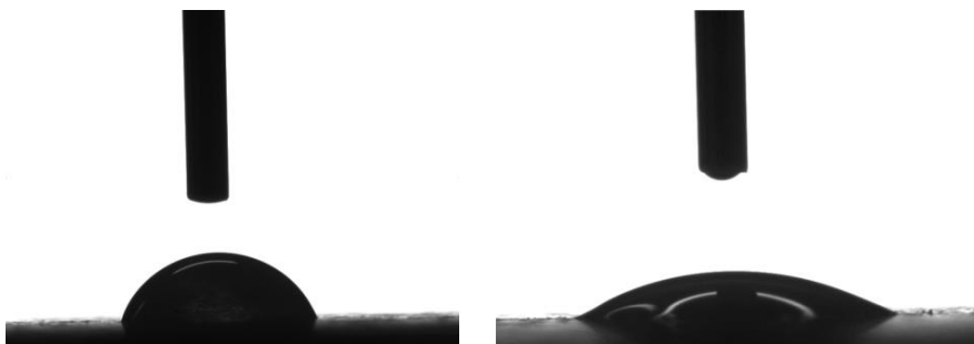
Fig. 6.1. Contact angle measurements for (left) before and (right) after irradiation with the UV lamp for 8h.
