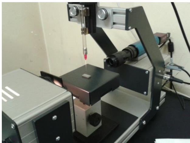
Fig. 3.8. Picture of water contact angle, model FM40Mk2 EasyDrop , KRUSS GmbH.
