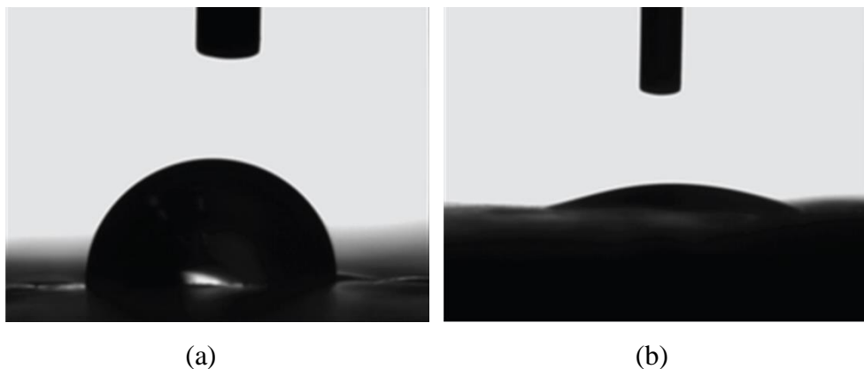
Fig. 3.22. Contact angle: (a) Orosei; (b) Orosei Active tiles.
