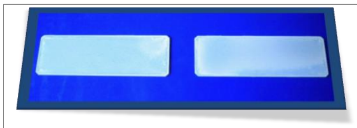
Fig. 4.1. TiO 2 powders catalysts deposited on glass laminas.
