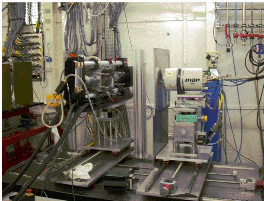
Figure 2.5: 2D-Diffraction setup on penta-pod table. In this experimental configuration the detector stage holds Mar133 CCD-detector and sample stage holds ETMT-rig. Al-plate before the detector cuts low energy fluorescence background and holds the beam-stop.
