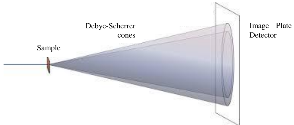
Figure 1.2: Diffraction cones produced by a sample in a X-ray diffraction experiment.
