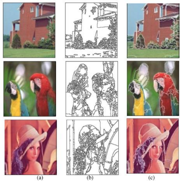
Figure 5. Image (a) shows the original, image (b) shows the over-segmentation with a traditional watershed algorithm, image (c) show Dombre's algorithm applied on image (a)
