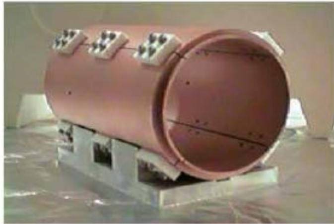
Figure 2.2 Picture of an azimuthally four sectored electrode, built of four insulated parts.
