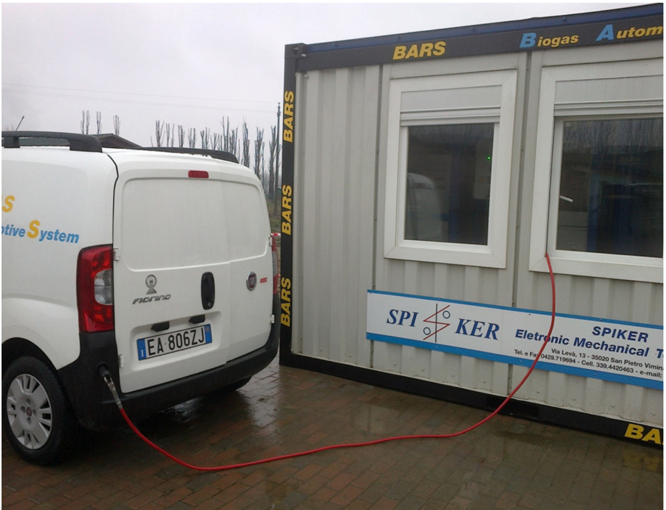
5.16: In situ -produced biogas fueled van.
