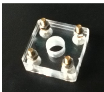
Figure 5.20. Experimental setup for the thermo-responsive characterization of hybrid PHEMA/PNIPAAm layers under mechanical constraint. a) Schematic view of the final assembly. b) Photograph of the PMMA jigs assembled together with M4 screws. c) Photograph of the compressed hybrid layer in the water filled Petri dish.
