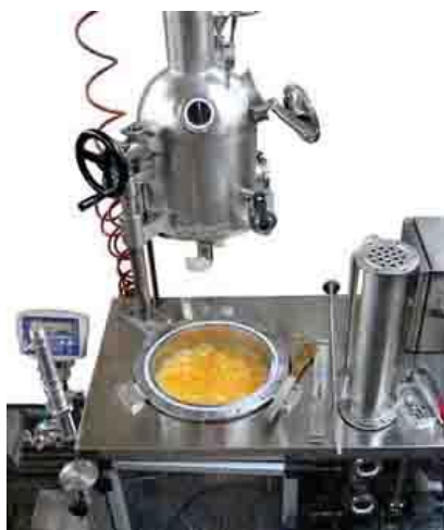
Fig. 2. The concentration boule in "open container" configuration.
