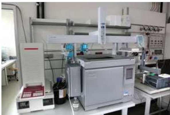
Figure 5.1.1 Coupled LC-GC system used at Fraunhofer IVV
