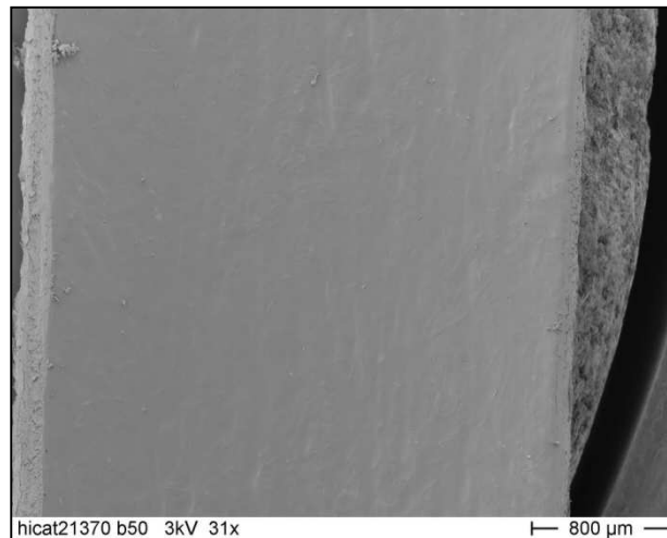
Figure 5.2.16 SEM observation for surface of coated Paperboard A (overview)
