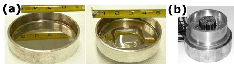
Figure 1.3: (a) Ferrofluids without (left) and with (right) an applied external magnetic field: controlling the magnetic field the mirror can assume the wanted shape (images from University of Laval). (b) Actuating mechanism of a ferrofluid based mirror: the magnetic field is modulated by a series of coils [33].
