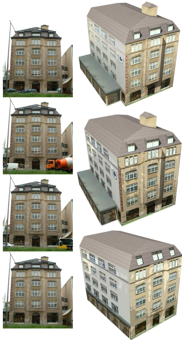
Figure 1: Left: Occlusion-free texture (bottom) by multiple image fusion. Right: Two abstraction levels (1 st image, 2 nd geometry) from a photo-realistic 3D building model (top).
