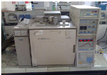
Fig. 4.12. Example of GC analysis for the quantification of heavy FT products
