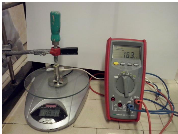
Figure 10.6.: Experimental set-up for the measurements of the resistivity variation during loading/unloading cycles (0-20 N).
