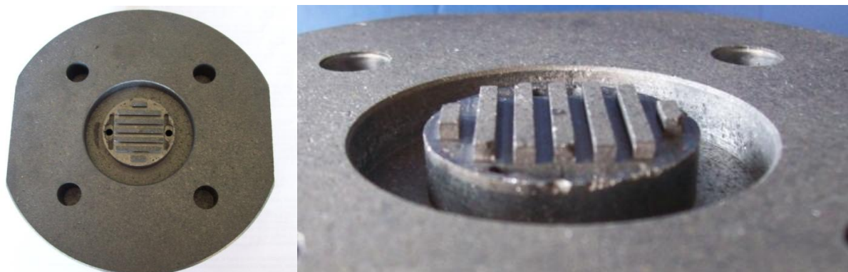
Figure 50: Graphite current collector used in the flux cell.
