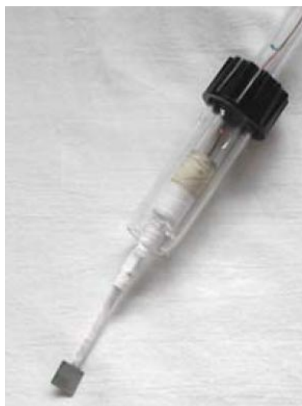
Figure 43: Ti plate support used for powders characterization.
