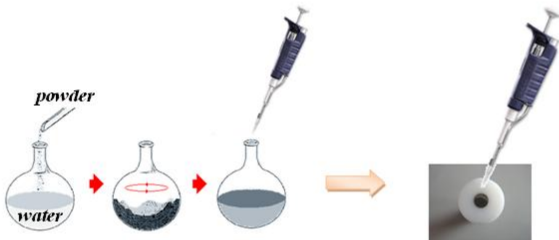
Figure 57: Schematic procedure for the modification of the rotating disk electrode.
