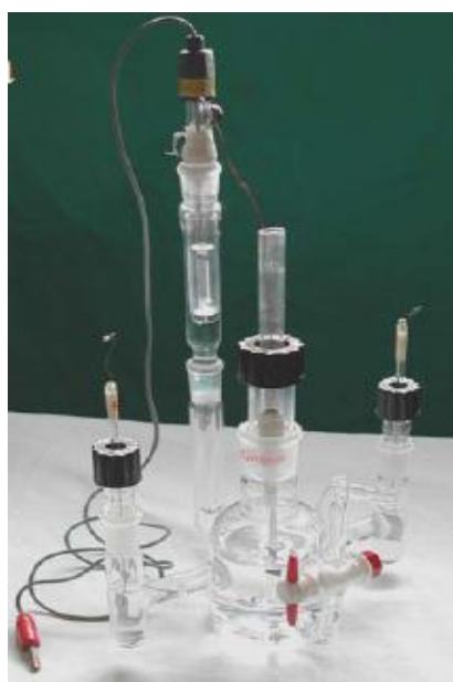
Figure 44: Cell used for electrochemical characterizations on Ti and GC supported powders.
