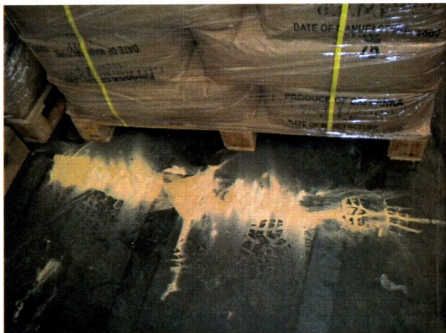
Figs 1 - 2. Fine dust ejecting from exit holes and accumulating below wood pallets.
