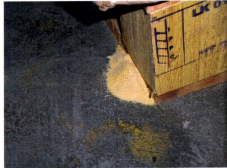
Figs 1 - 2. Fine dust ejecting from exit holes and accumulating below wood pallets.
