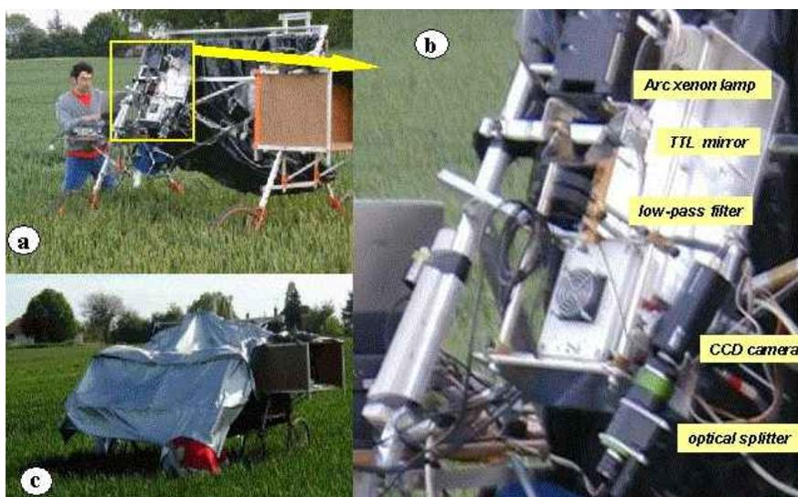
Figure 2. Set-up for field fluorescence imaging: (a) the MSFI mounted on the instrumented buggy; (b) the components of the imaging system; (c) the reflective shield reducing the disturbance of the environmental light on the sensed canopy.
