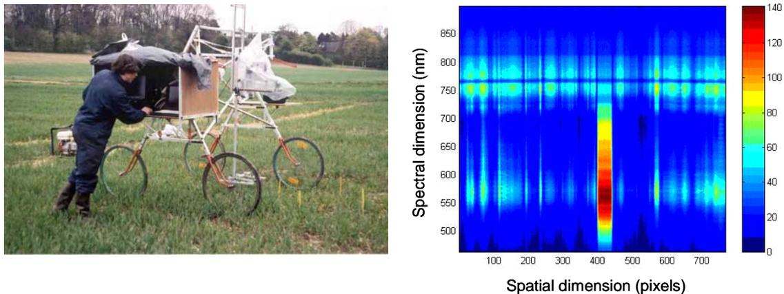
Figure 1. ( Left): The buggy on which the spectrograph was mounted. (Right): a spectral image as it was stored.
