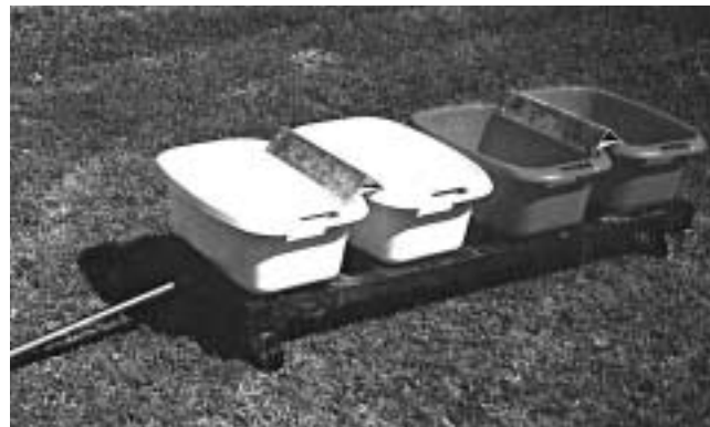
Figure 3—Four containers placed on a trolley made it possible to simplify the fertilizer-collection procedure for determining the flow rate.
