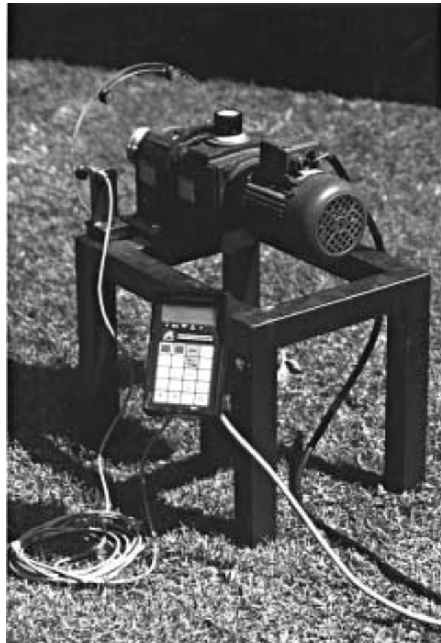
Figure 2—The electric motor-reduction gear group used to set the spreader work speed. The picture shows also the on-board computer of the tested system.
