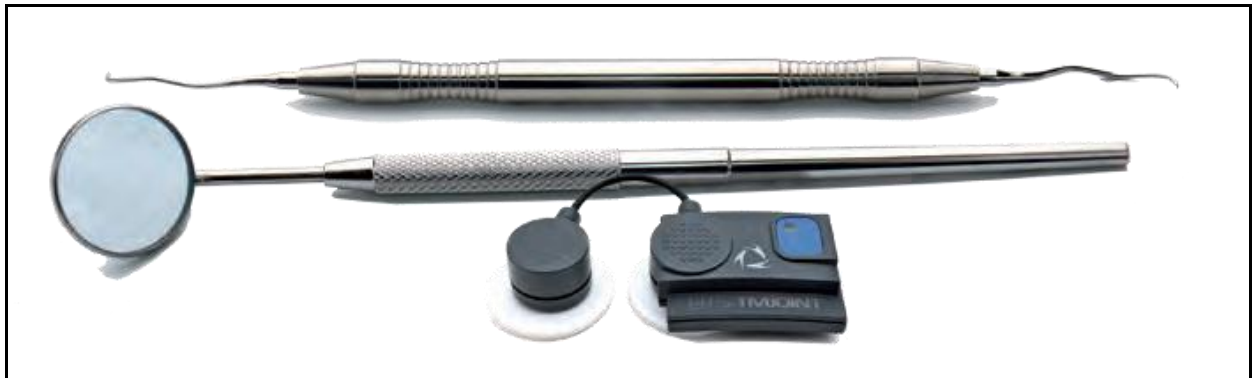
Figure 15. Detail of an EMG probe clipped on a pair of electrodes.
