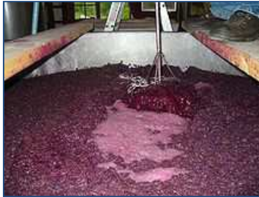
Figure 22: A cap of red grape skins in the fermentation tank (Font: www.wikipedia.org )
