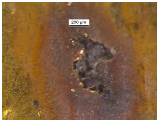
Figure 13: Sample E2 – stereomicroscope image of a detail of the golden surface (a) and of the cross section (b). A thick reddish layer of cuprite can be observed in deep respect to the surface.
