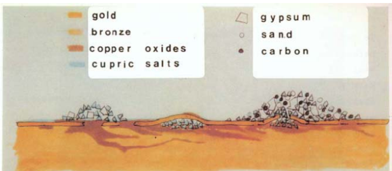
Figure 2: Schematic representation of the degradation products distribution and the deposited materials on the surface of the Porta del Paradiso [5].
