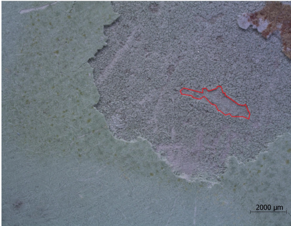
Figure 13: Evolution of the growth of the second layer of corrosion products: compact layer on the top and powdery part (circumscribed by a red line).
