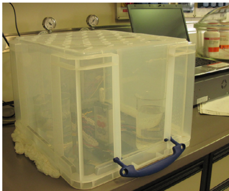
Figure 4: Setup for the increasing relative humidity experiment.
