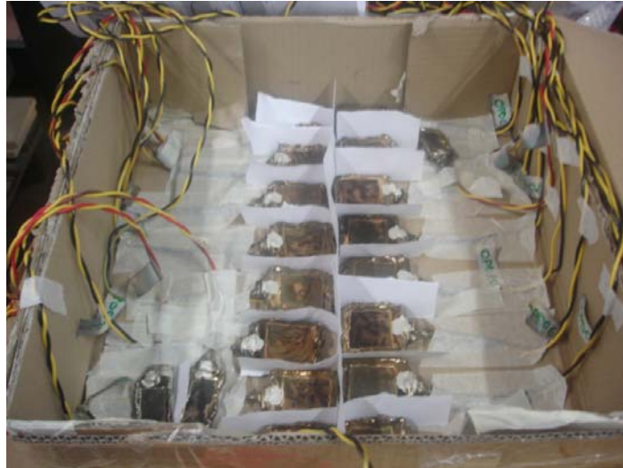
Figure 1: Galvanic sensors at the OPD laboratory, during the preconditioning period.
