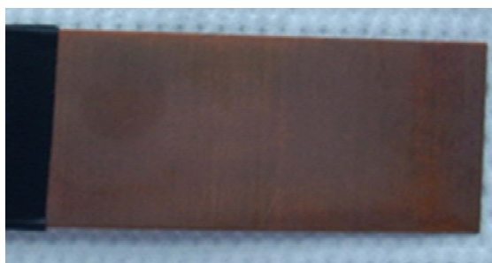
Figure 1: Layer of cuprite on copper prepared following recipe 3.3 [2].
