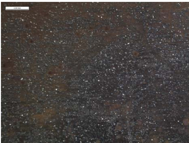
Figure 6: Macro (a) and stereomicroscope (b) (c) images of the dark patina formed on the sample treated with “wet and dry” procedure in artificial rain for 3 weeks.
