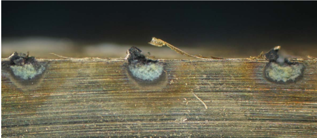
Figure 19: Cross section stereomicroscope image of sample S2 in which the scratches of Figure 32 are visible (2,5X magnitude).
