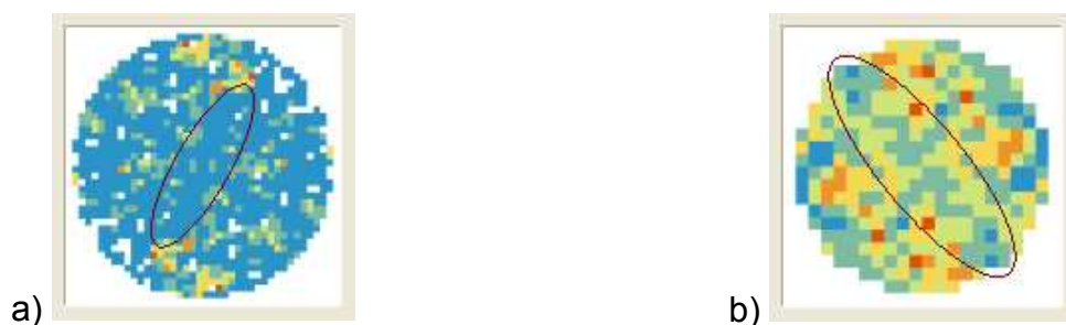
Figure 5: 2D variogram maps of: horizontal intercept (a) and J_v transformed data (b)
