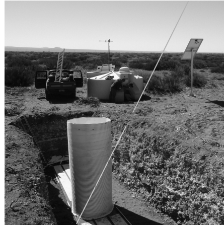
(b) The detector concept: a muon of sufficiently high energy is capable of reaching the buried scintillator.
