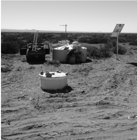
(a) Surface infill SD station with its associated muon counter already buried.
