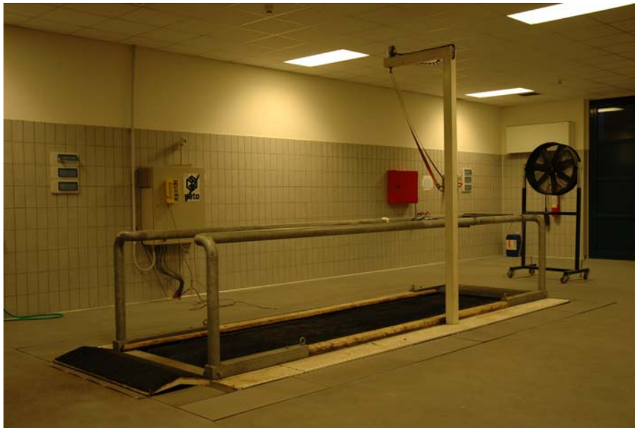
Figure 3: High speed treadmill in a dedicated room with controlled environment
