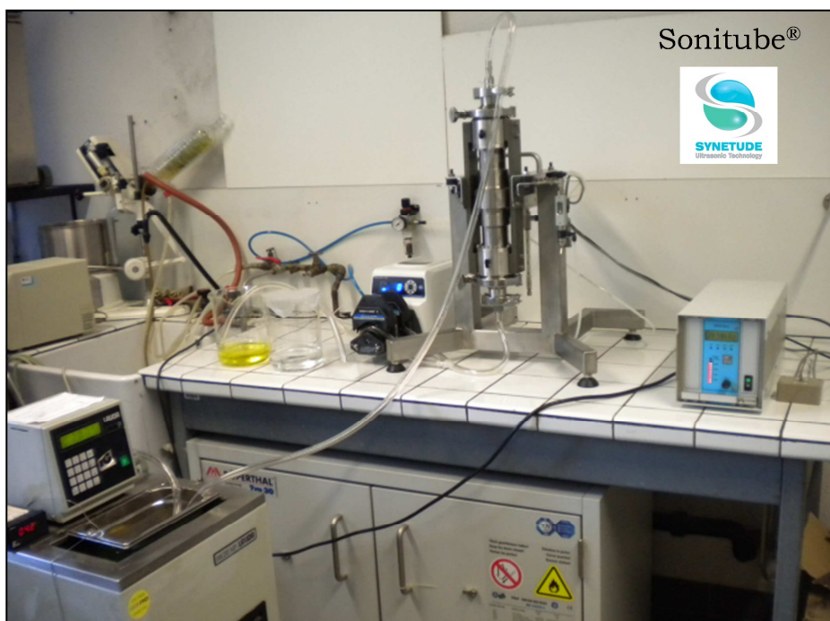
Fig. 8.3. Continuous reactor Sonitube® (Synetude Company – Chambery, France): V = 0.700 \text{ L} .
