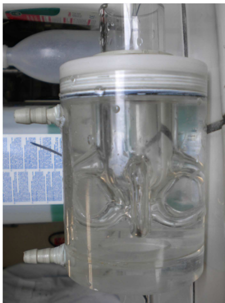
Fig. 8.1. Rosett cell reactor.
