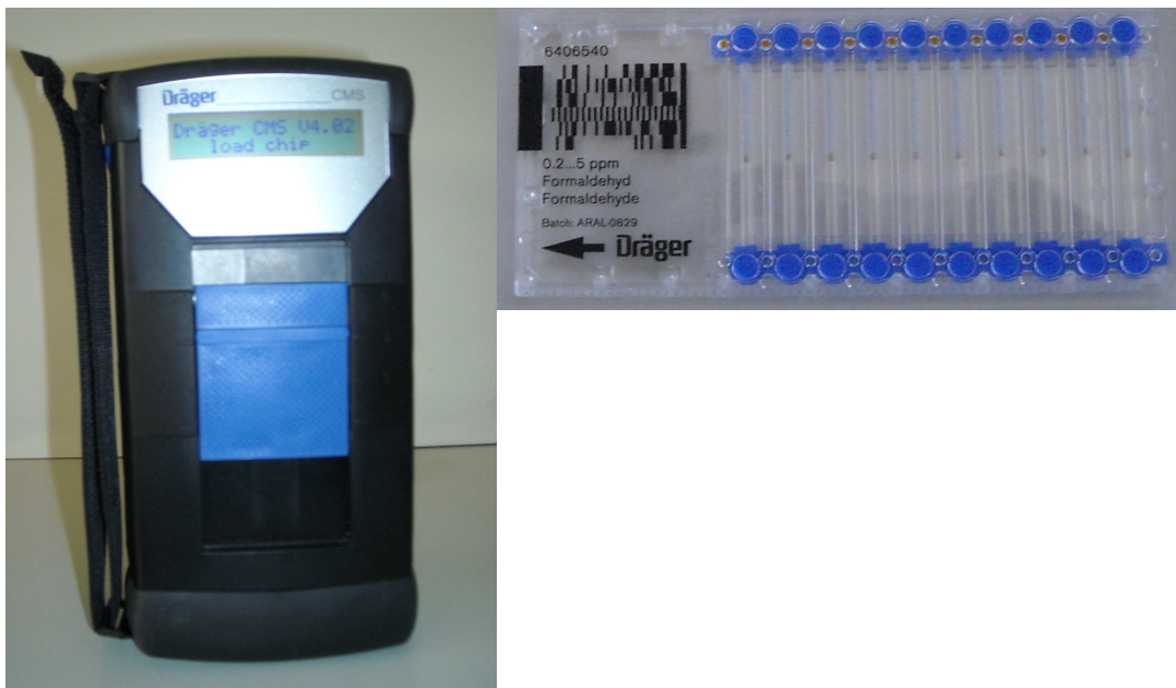
Figures 2.2.2.3a and b. Active sampler Dräger CMS and chip containing 10 micro- vials.
