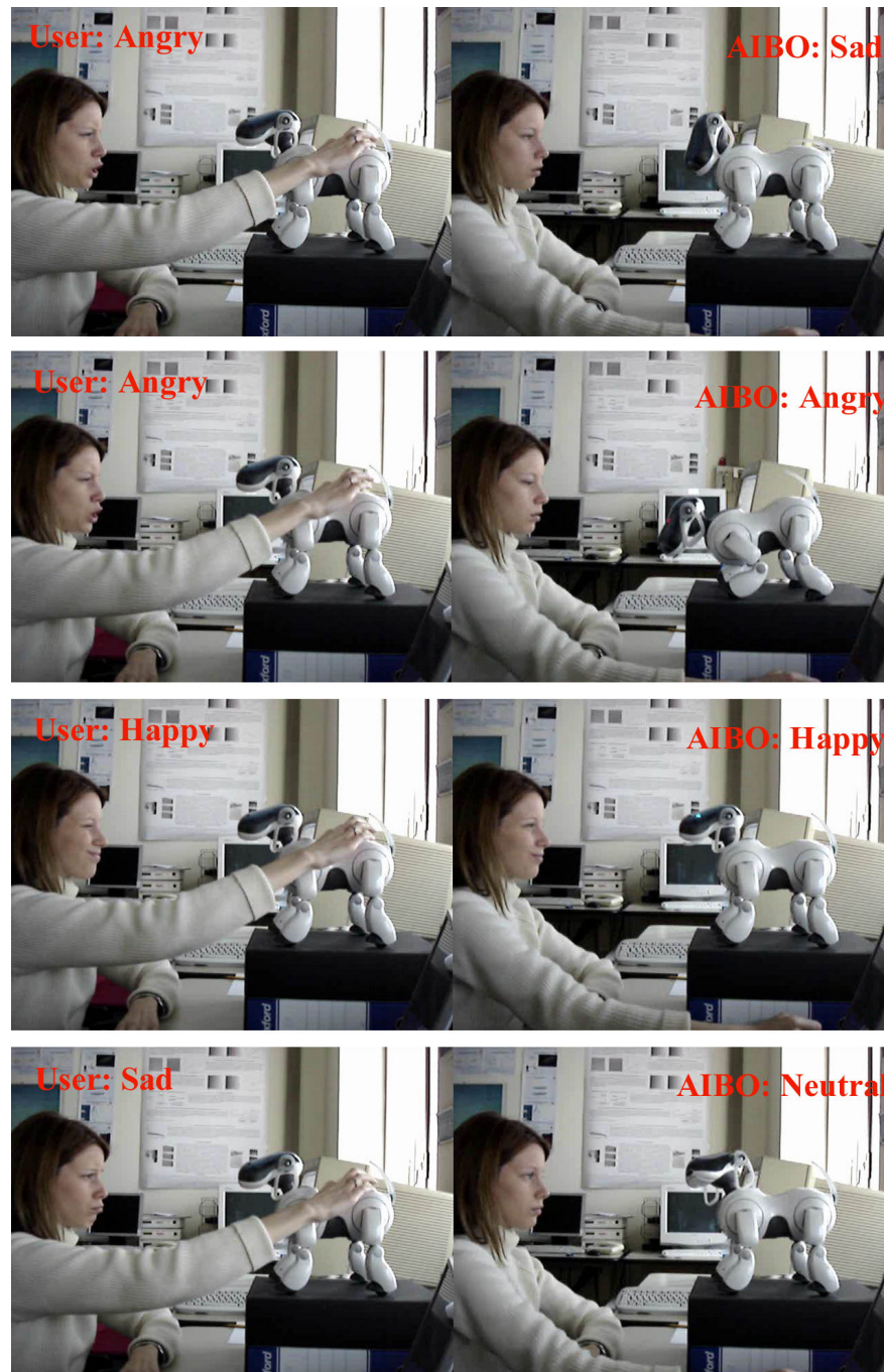
Figure 8.2: Four phases of an emotional interaction with AIBO. In the left panels, the emotional expression displayed by the master. In the right panels, the emotional response of AIBO. In particular, the sad expression is displayed by AIBO lowering its head and playing a sad melody; in the angry expression AIBO moves quickly forward in an aggressive fashion and growls, while in the happy expression the robot wags its tail and barks happily. In the neutral expression AIBO stands still, looking around as if it is uninterested in the user.
