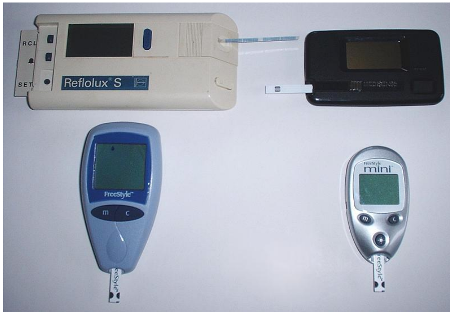
Figure 19. Four generations of blood glucose meter, ca. 1993–2005. Sample sizes vary from 30 to 0.3 \mu l.
