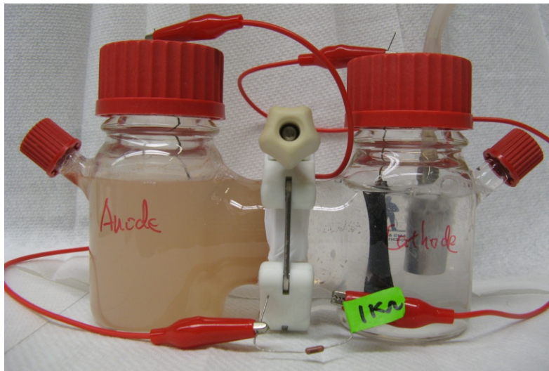
Figure 47. A set of lab scale classic H-shaped two-chamber MFC. Anode is CNT-cotton and cathode is carbon cloth with a platinum catalyst layer. Anode and cathode chambers are separated by an ion exchange membrane. Domestic wastewater is used as the inoculum. Anode is fed with glucose and cathode chamber is continuously purged with air using a diffusion stone. The loading is a 1 k \Omega resistor. The turbidity in the anode chamber (left) is caused by the growth of microorganisms.
