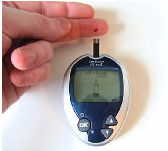
Figure 18. Blood glucose testing, showing the size of blood drop required by modern meters.
