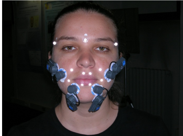
Figure 14. Position of the reflective markers and the electrodes of the BTS FREEEMG system (BTS S.p.a, Garbagnate Milanese, Italy).
