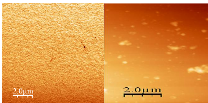
Fig. 43 AFM images of mesoporous titania thin films before (left) and after (right) the functionalization with APTES
