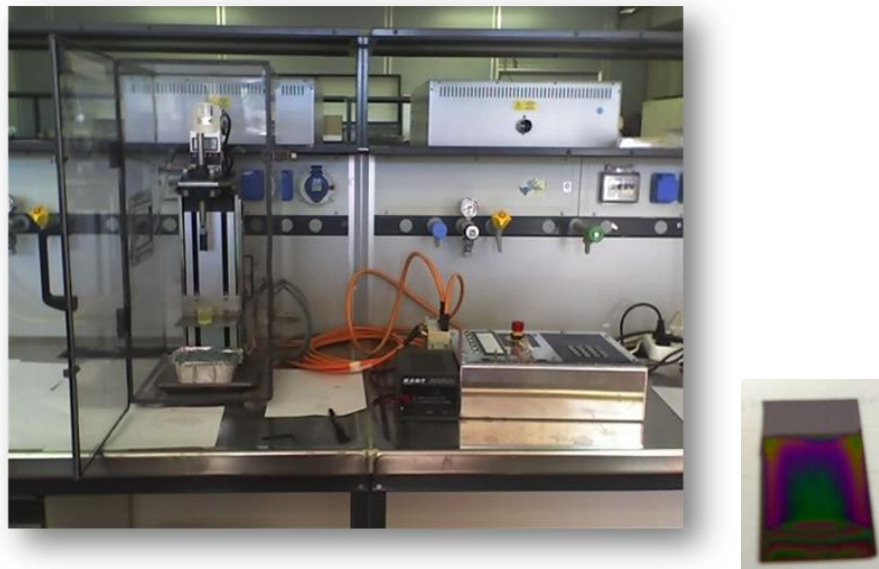
Fig. 15 Picture of the home made dip-coater used in the present work (left), and the deposited thin film on Si (right) .
