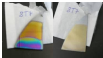
Fig. 77 Picture of titania thin films before (left) and after (right) UV exposure for 6h
