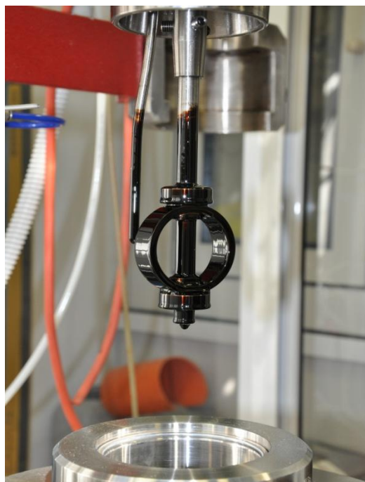
Figure 2.5 – HT-HP specimen mounted in the autoclave
