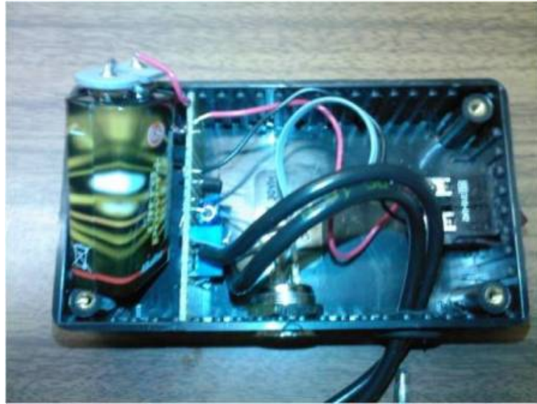
Figure B.7: A picture of the low-cost homemade gaussmeter.
