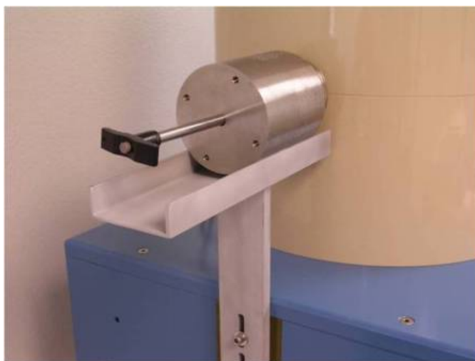
Figure 2.2: The source holder. The cylinder in the background is part of the moderator system.
