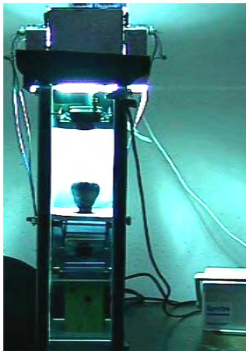
Figure 1. The experimental fluorescence imaging system. Two actinic sources were tested on red-pigmented cultivars of apple and peach fruit: a filtered UV-blue lamp (360–570 nm) and an array of ultra-bright red LEDs (630–670 nm).
