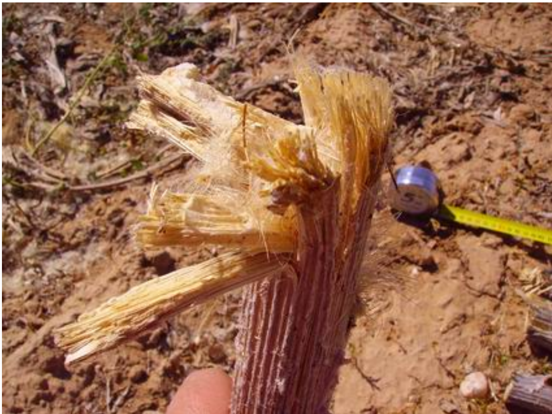
Fig. 23. Rotating blades scraped cut.
