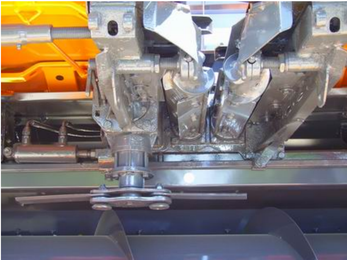
Fig. 3. Squeezing rolls, adjustable detaching plates and rotating blades.
