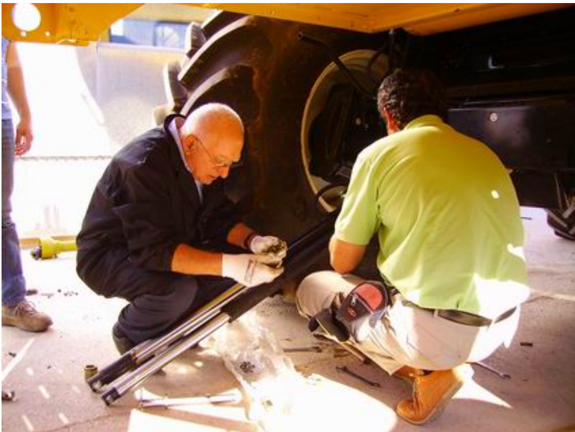
Fig. 16. Third hydraulic cylinder installation.
