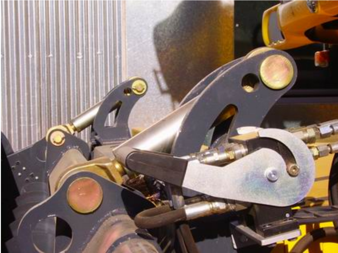
Fig. 12. Tilting device and hydraulic quick coupler.
