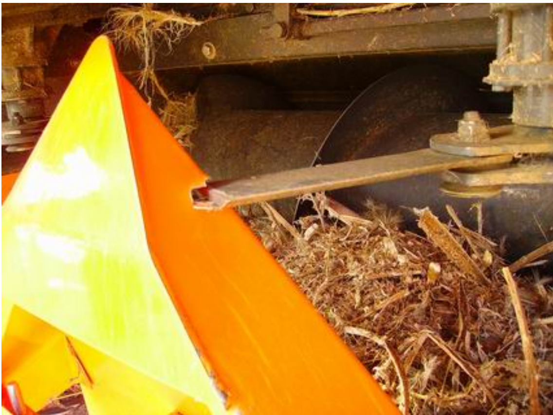
Fig. 22. Lower divider hit by rotating blades.
