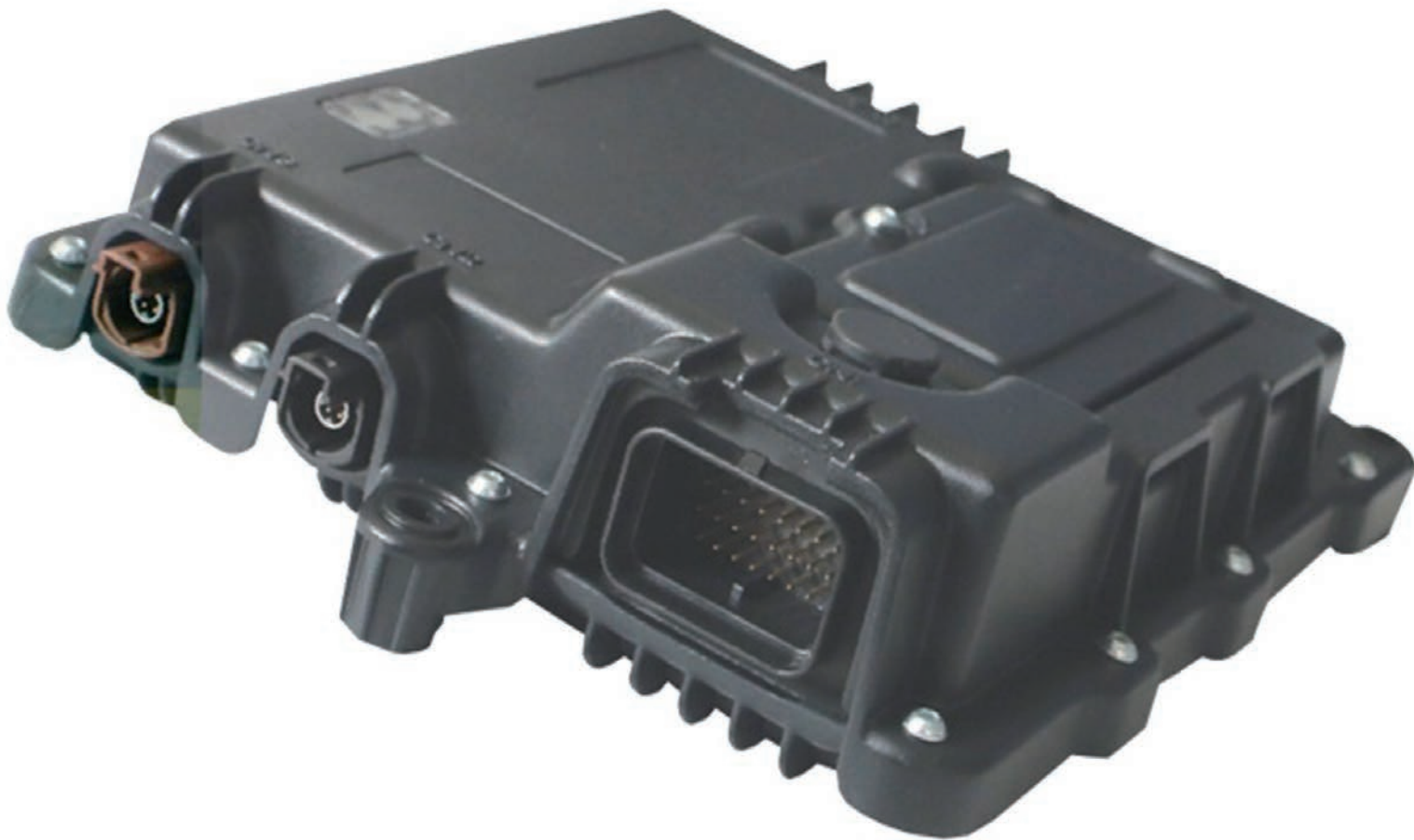
Centralina elettronica TGU-R di Actia per applicazioni di telemetria remota installata su trattori McCormick (da: https://www.actia-pcs.com ) Actia TGU-R electronic control unit for remote telemetry applications installed on McCormick tractors (from: https://www.actia-pcs.com )
