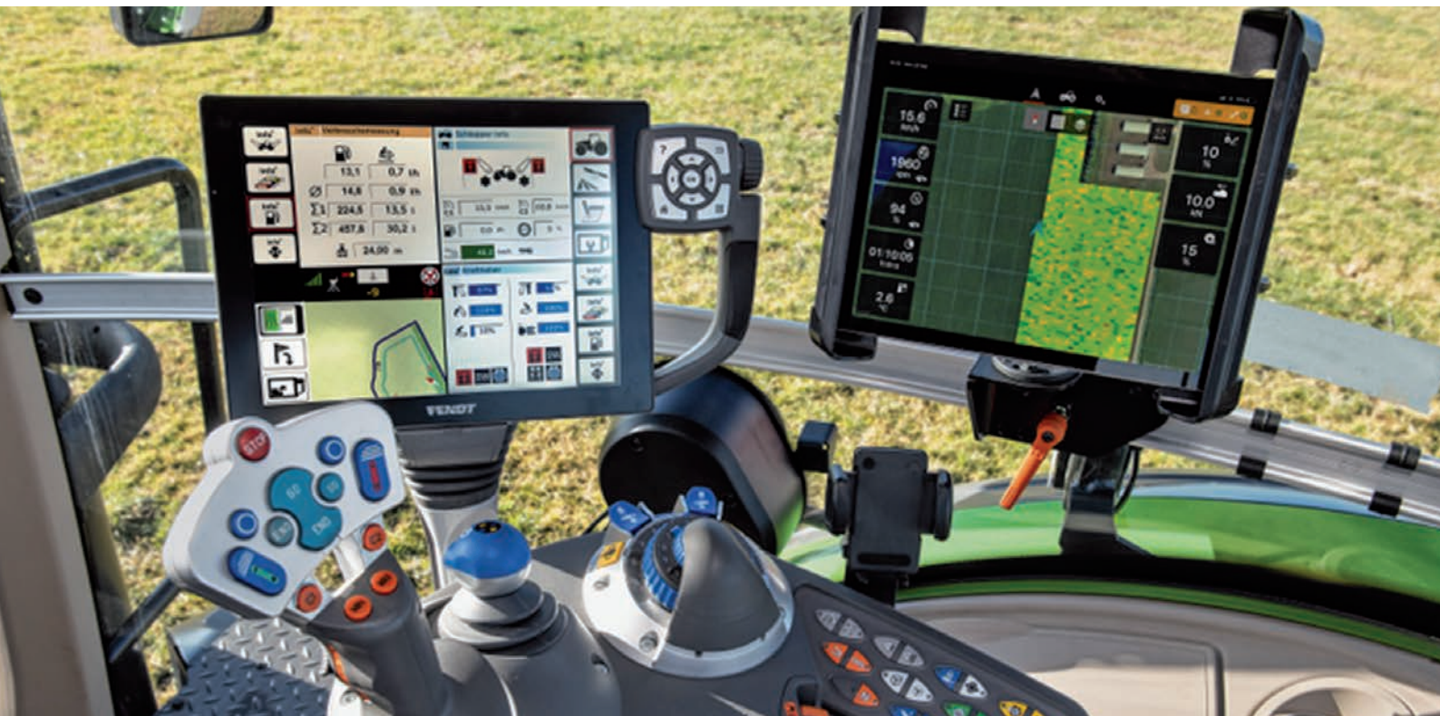
Interfaccia di bordo del sistema Fendt Connect che consente, oltre al monitoraggio operativo, l'assistenza remota del mezzo (da: https://www.fendt.com ) On-board interface of the Fendt Connect system that allows, in addition to operational monitoring, remote assistance of the vehicle (from: https://www.fendt.com )
