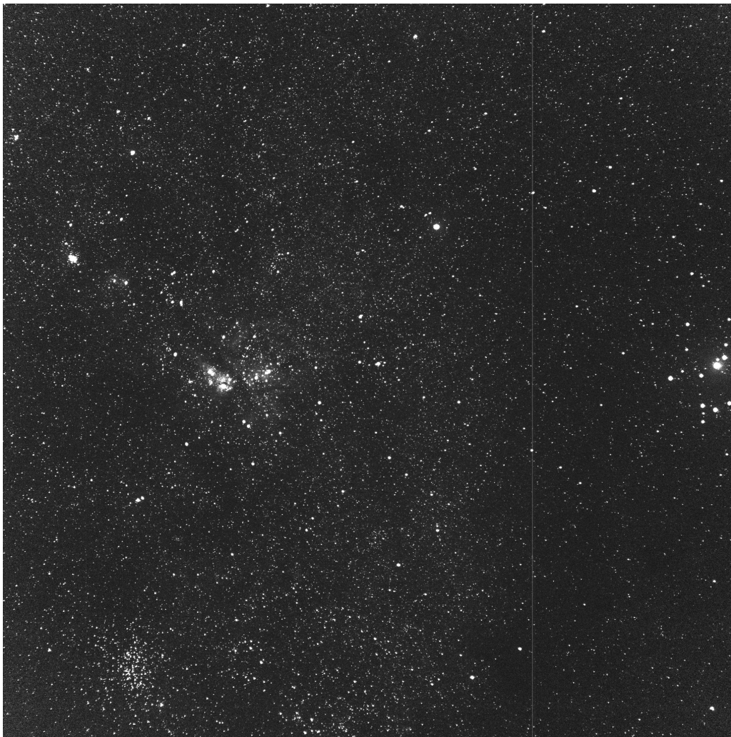
Figure 3. One of the images taken by the Auger FRAM during a Mode A altitude scan, in this case covering a well-known region of the Milky Way around the star \eta Carinae and its surrounding nebula (seen left of the center). A single 30-second exposure in the Johnson B filter can be used to measure the brightness of hundreds of stars simultaneously in such a rich area.
