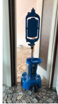
Fig. 7: The robot dealing with a narrow passage, a door that can be only partially opened due to furniture behind it.
