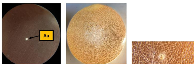
Figure 5.11 - Cross section of Au disk microelectrode before (left) and after (right) dip-coating in \text{TiO}_2 sol.
