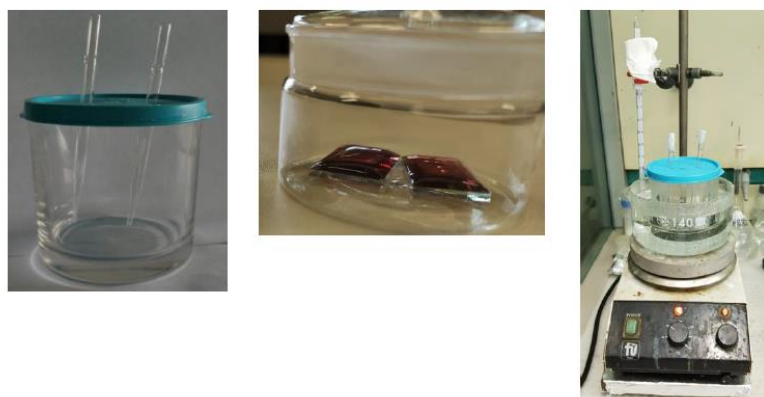
Figure 2.30 - the image on the left is the cell created ad hoc, on the right there is the global system to perform the synthesis of the slides, at the centre is the deposition of gold nanoparticles on the electrodes.
