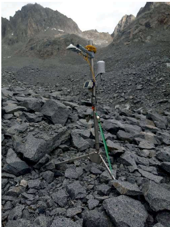
Fig. 2. The weather station on Amola glacier AWS_{Amola} . Typical clast size of supraglacial debris is also shown.
