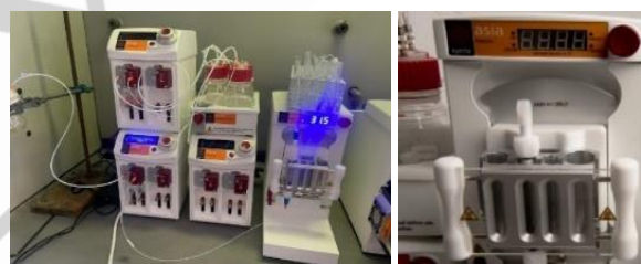
Figure 4. Packed bed reactor in the Asia Syrris Premium system.
