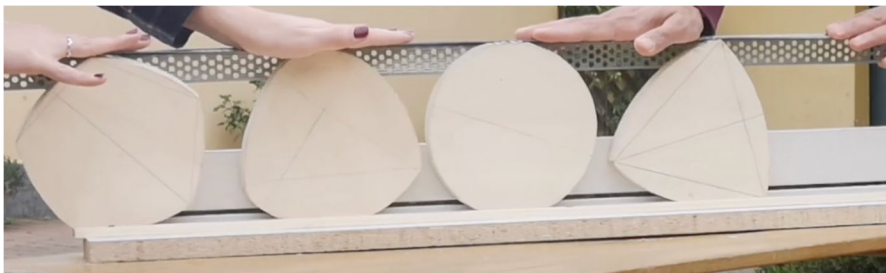
Fig. 11 Reuleaux triangle and other constant-width shapes as wheels (frame taken from the video https://www.youtube.com/channel/UCXWF_gKgyUXVSK3t35SdjFA )
