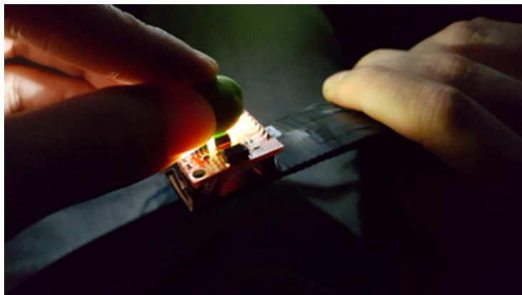
Figure 1. First version of a simplified LED prototype during optical acquisitions on olives.
