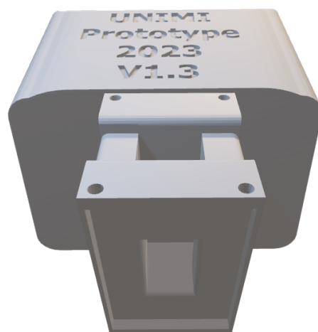
Figure 4.5.2 Main case and cuvette holder of the prototype.
