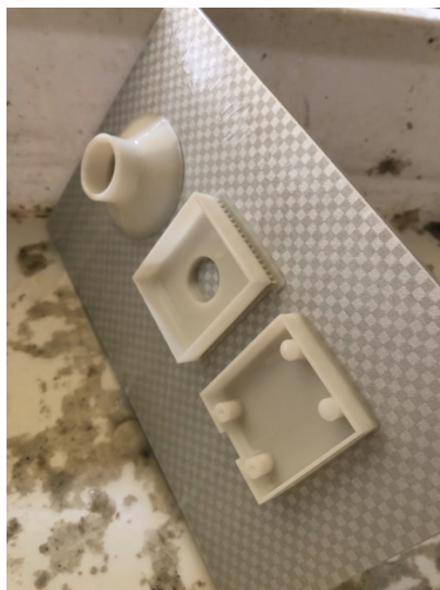
Figure 4.7.2 3D printed parts of the prototype.
