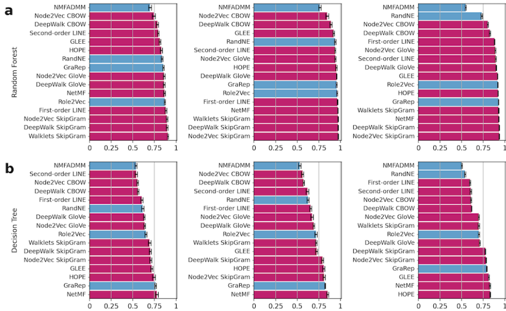
Figure F.8: Average auroc of node label prediction models trained on embedding methods. Results are averaged across ten holdouts. Embedding models are sorted for each task; methods implemented in GRAPE are in purple, while methods integrated through the GRAPE interface are in cyan. We show random forest and decision tree in row a and b , respectively. From left to right, CiteSeer, Cora and PubMed Diabetes datasets..
