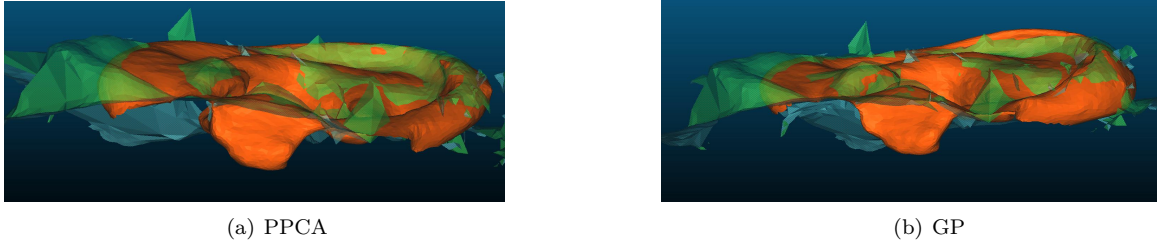
Figure 4.13: Detail of shape completion step with PPCA and GP for the same sample. The green shapes correspond to the original scan and the orange ones to the shape predicted by each approach. Looking at the small protuberance on the bottom of the ear, it is clear that the PPCA model does not have enough variability to properly deform the template. On the other hand, the augmented kernel of the GP is able to provide the necessary variability, when given the same correspondences as the PPCA model.
