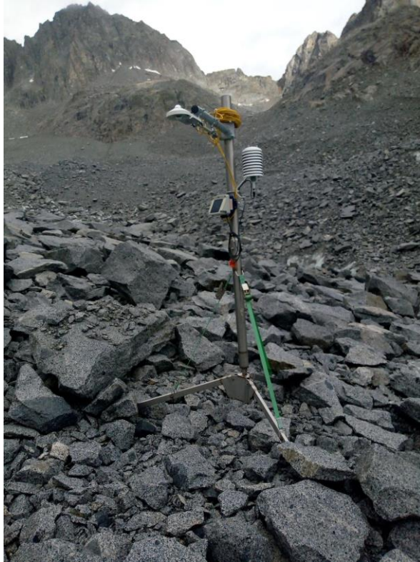
Figure 2: The weather station on Amola glacier AWS Amola . Typical clast size of supraglacial debris is also shown.
