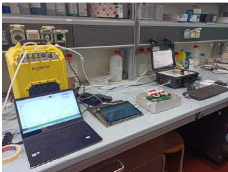
Figure 2. Calibration setup used for \text{NH}_3 and \text{H}_2\text{S} sensors.
