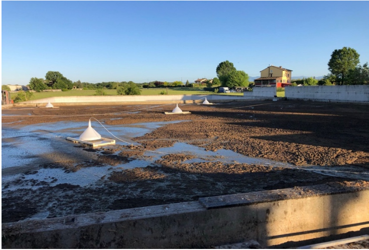
Figure S5 - Floating PVC funnels placed on the slurry surface in one of the slurry storages during the measurements.
