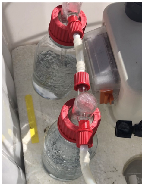
Figure S1 - Detail of one of the acid traps used to detect ammonia emissions. In the photo it is recognizable that the solution is bubbling due to the passage of the air sucked in by the vacuum generated by the pump
