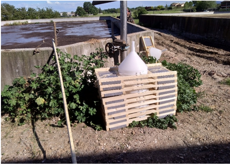
Figure S3 - Close up of the floating PVC funnels used for setting up the measurement system.
