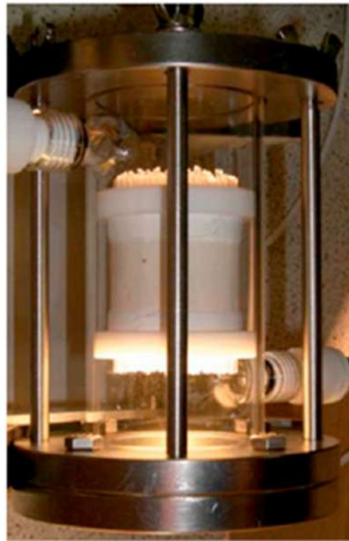
Figure 16. Internally illuminated monolith photoreactor: optical fibres are embedded within the monolith to improve light penetration through the solid support. Reproduced by kind permission of RSC from [109].
