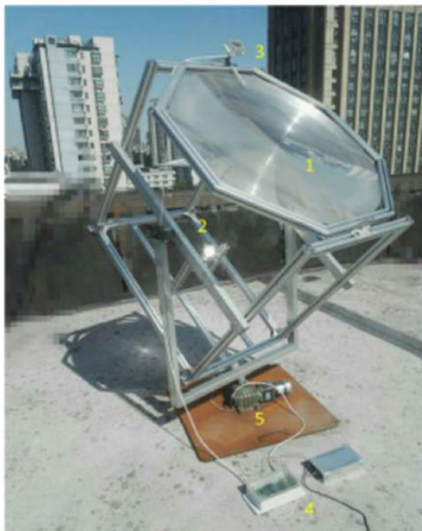
Figure 29. The concentrating reactor system. 1. Concentrating mirror; 2. Reactor; 3. Sensor for tracing sun; 4. Controller; 5. Motor. Reproduced by kind permission of Elsevier from [168].
