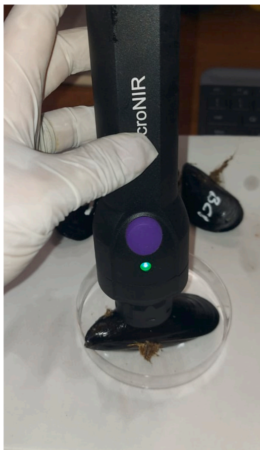
Fig. 1. Acquisition of NIR spectra using the portable instrument through the shell of live mussels to predict the storage time.
